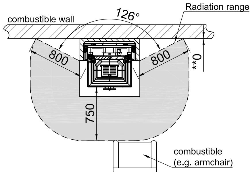
\*\* Using a heat protection plate
