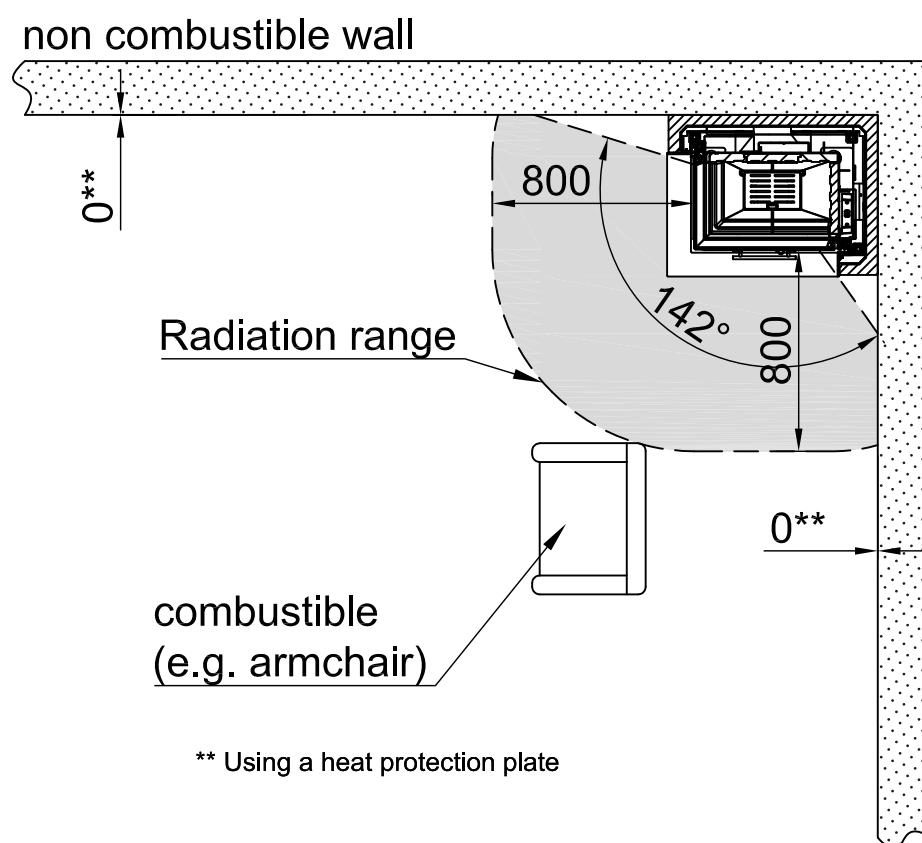
\*\* Using a heat protection plate
